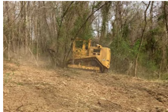
Figure 15 Forestry mulcher in action
