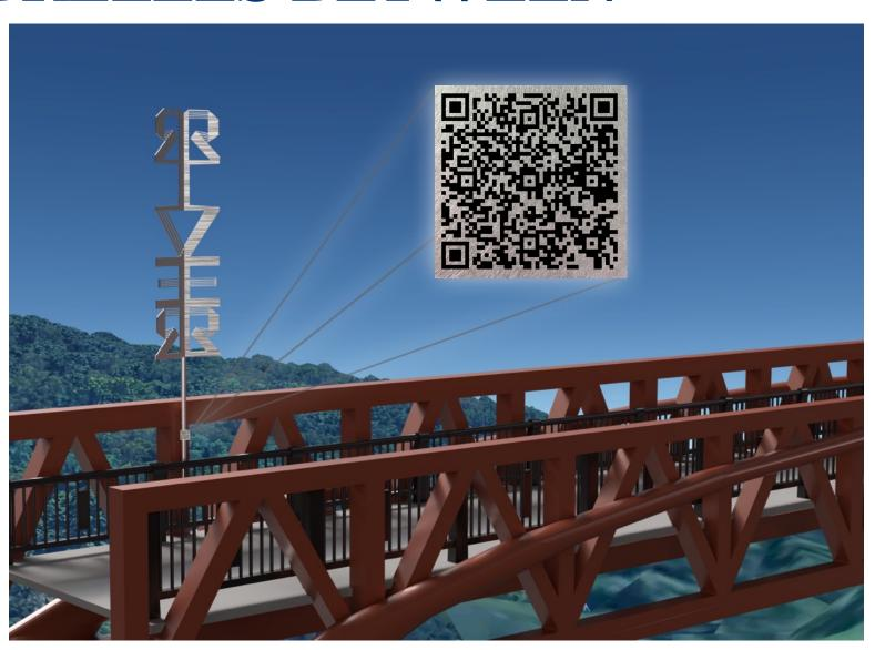
The QR Codes will be CNC milled out of Stainless Steel with the raised areas treated with black finish.
